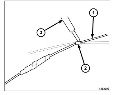
16. Center the heat shrink tubing (2) over the solder joint and heat using a heat gun. Heat the joint until the tubing is tightly sealed and sealant (1) comes out of both ends of the tubing.
